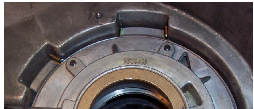
Completed installation, protects all four of pump tabs' cavities
