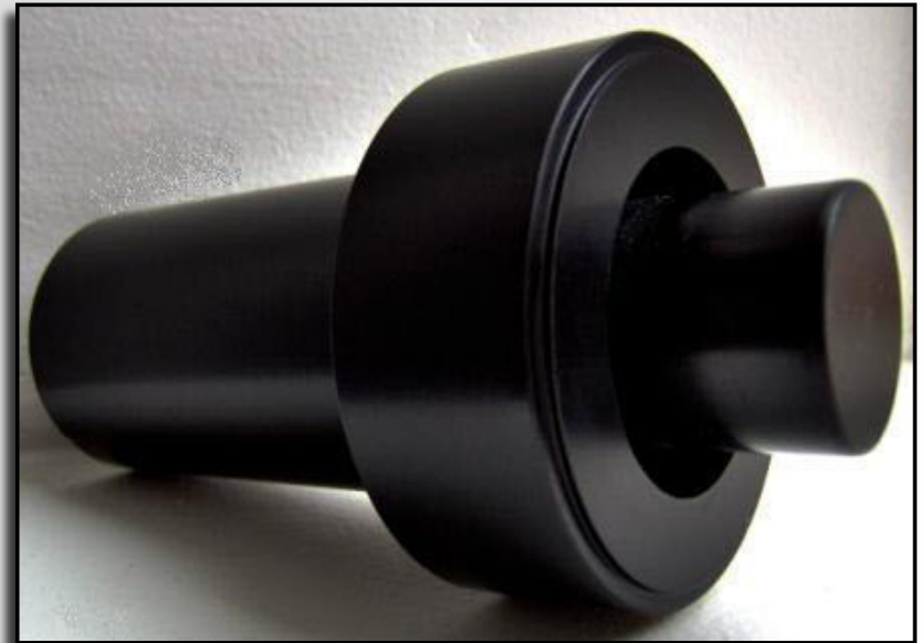
▼ Seal, for visual reference; note the two driving surfaces
