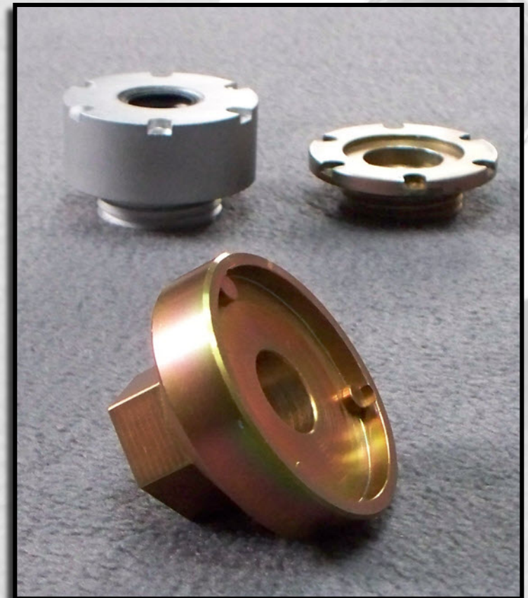
Pictured in the background are the two supports you'll find. The taller is for NP271 (manual), other used on electric NP273
