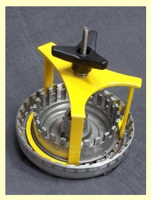
Recognize this drum? Nothing to fear as the Drum Buddy "I" is here. Note the ease of access to the snap ring. Also visible is the heavy duty ball bearing beneath the knob.
